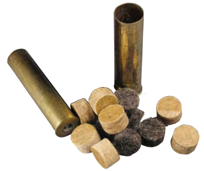
Felt does not fray and so can be die-cut for machine parts. Felt production peaked during the Second World War, when it was used in the manufacture of armaments and ammunition, including as wadding for shells.
